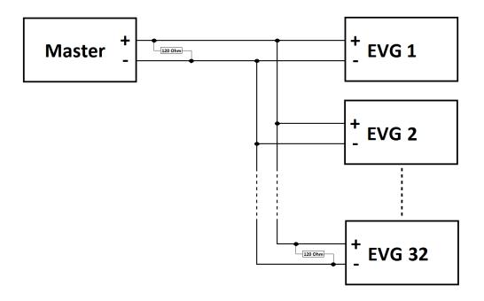
It is the use of a twisted pair cable recommended. Furthermore a bus termination should be used. This is done with a 120 Ohm resistor at both ends of the network (see connection diagram).
